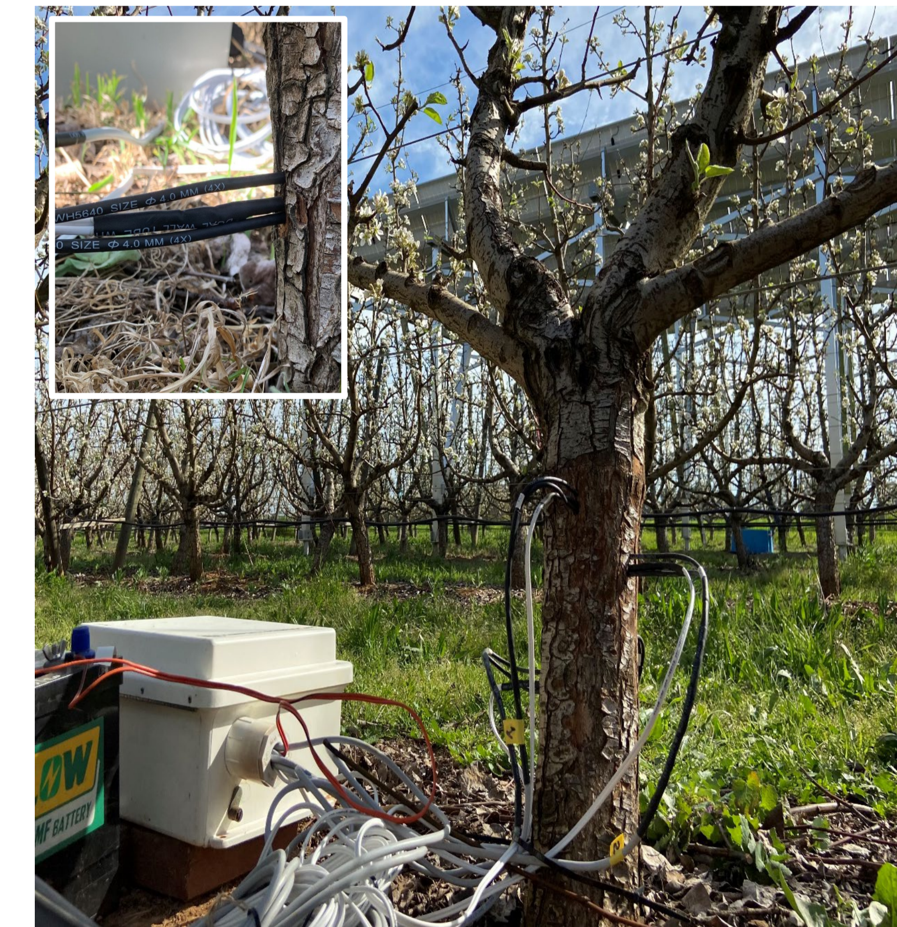
Four HPV sap flow sensors were installed per tree in 2 trees per treatment.
