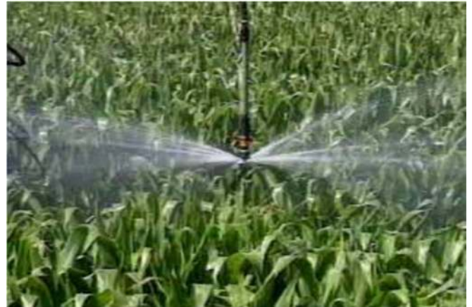
Figure 1: Moving plate sprinkler nozzle. (Picture source IAL CPLM course manual, 2010)
